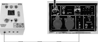
The ATS contact socket is located on the control panel of the generator.
