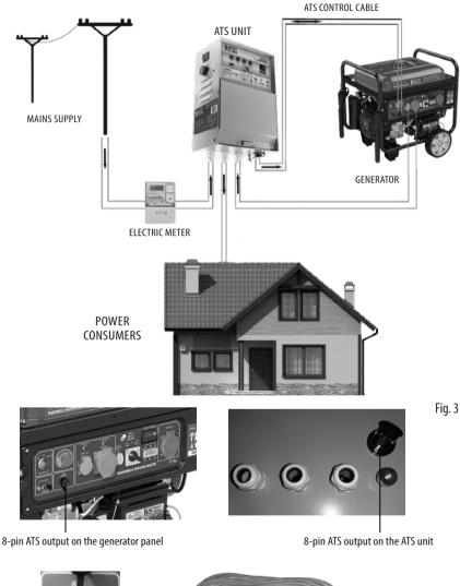
The ATS socket is located on the generator panel. Connect the ATS unit to the ATS input on the generator panel using the control cable (included).
