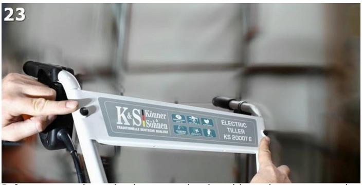
Before you start the engine, be sure to plug the cultivator into a power outlet. Press and hold down the blue button while lifting up the blue lever, as shown in fig. 24.
