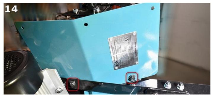
Use the two bolts to secure the console of the control panel, as shown in fig. 15. For the convenience of the user, the console can be adjusted in 3 positions.
