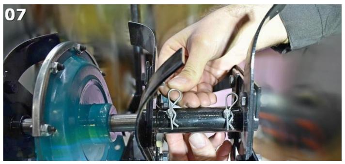
Put on the protective side disc, as shown in fig. 8.
