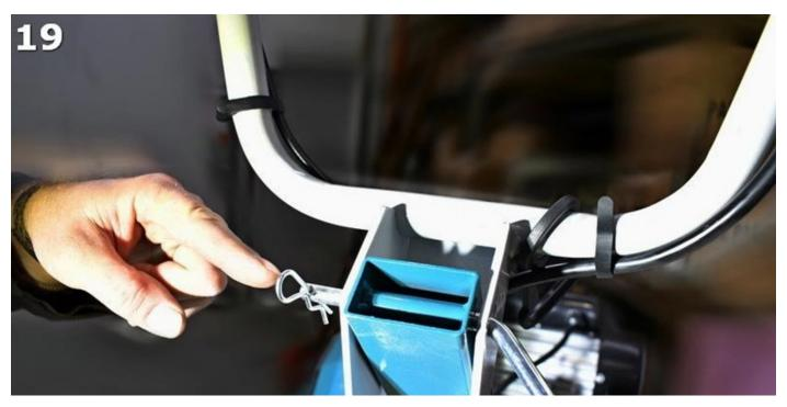
Fix the control panel in the lower position with the bolt, as shown in figs. 20 and 22.
