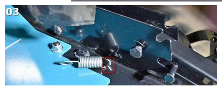
Use the pliers to grab the other end of the spring and fasten it to the special mounting screw on the transport wheel, as shown in fig. 4.
