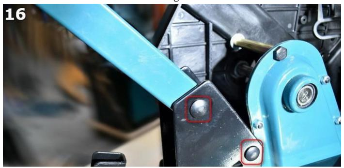
Install the operator's control panel using the bolt and locking bolt with cotter pin, as shown in fig. 17
