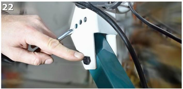
Install the decorative panel on the control panel with the two bolts, as shown in figs. 21 and 23.
