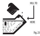
Recommended motor oil: SAE 10W30, SAE 10W40. Recommended motor oil grade: API Service SG type or higher. Motor oil quantity: see specifications table.
