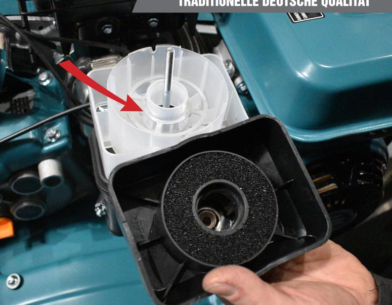
2) Fill 50-100 ml of engine oil into the air filter separator.
