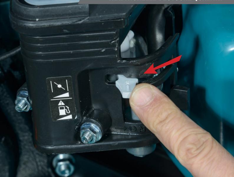
4. Turn the air choke control knob to "Closed".
