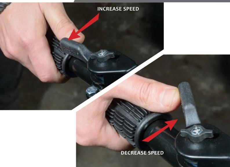
4.Use the engine speed control to adjust the speed.
