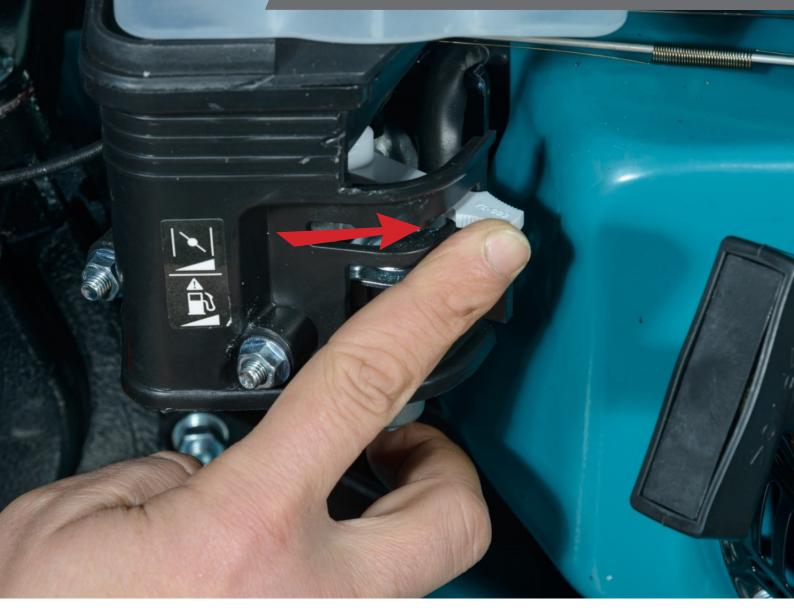
8. After the engine has started, turn the air choke control knob to "Open".
