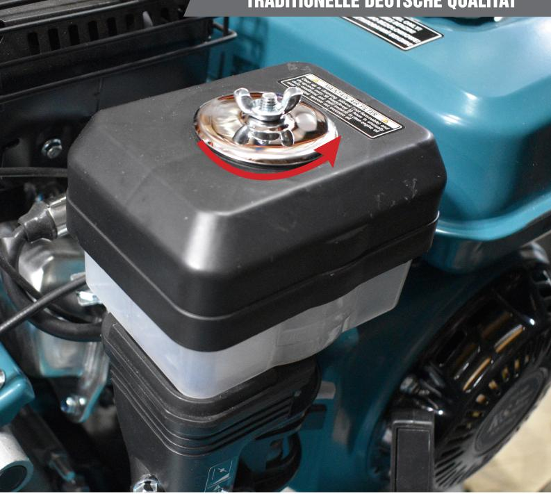
4. Preparing the air filter for operation1) Unscrew the air filter cover.
