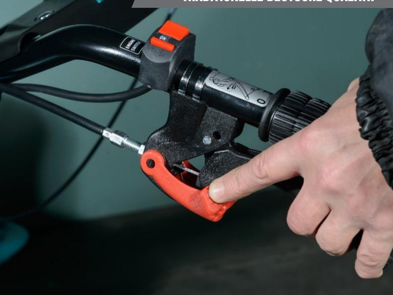
2. Gently press the red fuse (near the clutch lever), press and hold down the clutch lever.
