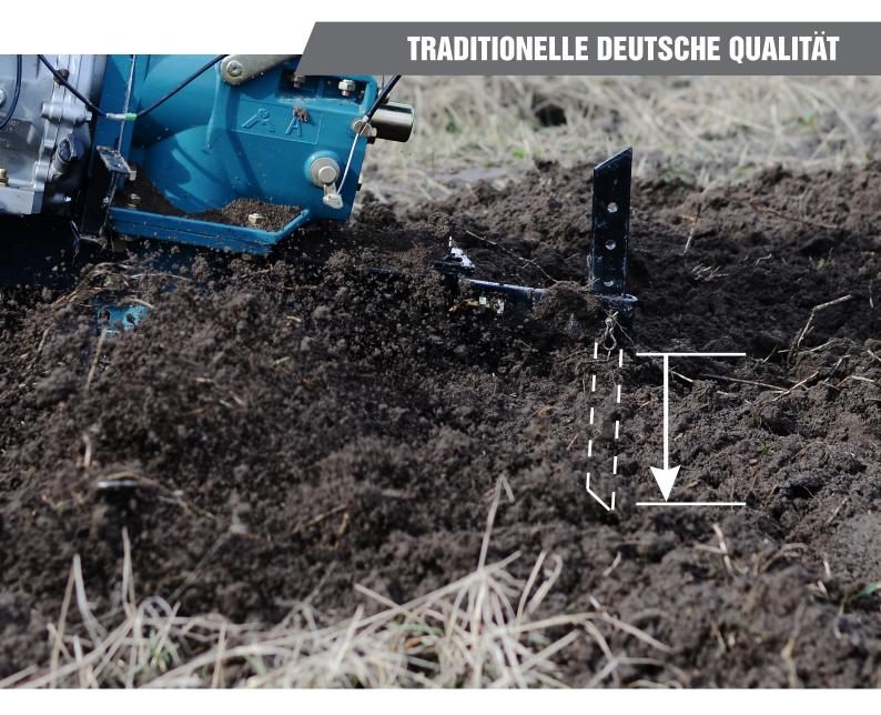
3. Gradually increase the tilling depth when cultivating soil, for which purpose apply pressure on the steering wheel to increase the coulter depth.
