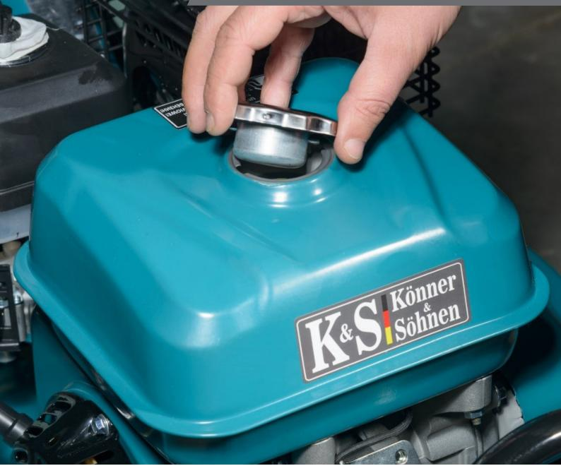
3. Fill the fuel tank with gasoline.
