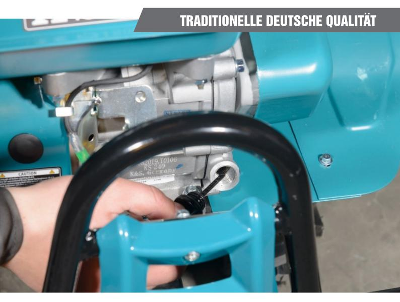
2. Fill the crankcase with engine oil.
