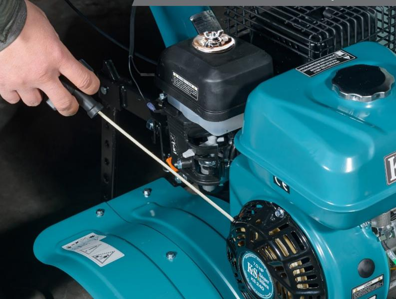
7. Pull the manual start cord to the full length with a sharp movement
