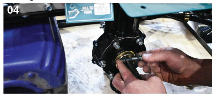
Fig. 5. Install the plow holder mount on the cultivator frame with the locking pin. Secure the locking pin with a cotter pin.
