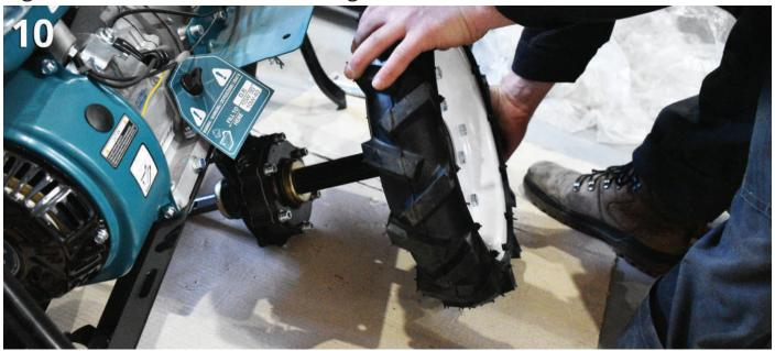
Fig. 11. Fix the wheel semiaxle to the gearbox shaft using a locking pin and a cotter pin.
