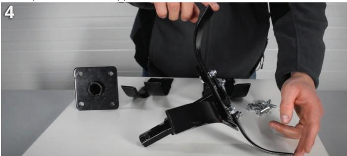
Fig. 5. Attach the 2 right knives to the inside of the base so that the bends point to the right opposite each other. The cutting edge of all knives should be at the front (in the direction of travel of the cultivator).
