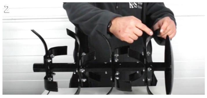
Fig. 3. Assemble the cultivator's left cutters. The left knives have their cutting edge against the user pointing to the left, with the right knives having their cutting edge against the user pointing to the right.
