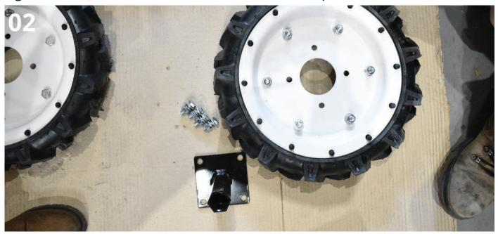
Fig. 3. Secure the transport wheel to the axle using a bolt, nut and washer.
