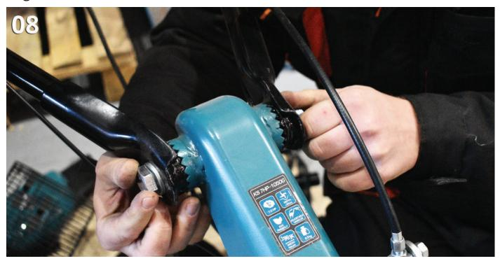
Fig. 9. Lock the position of the handlebars with the clamp fixture.
