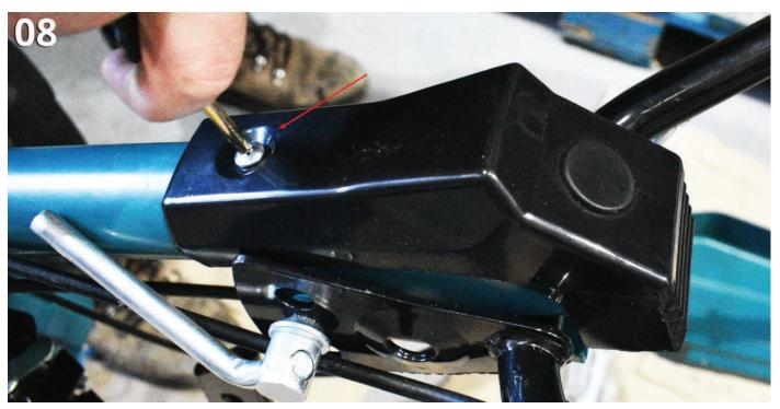
Fig. 9. Secure the fender to the cultivator with bolts and nuts.
