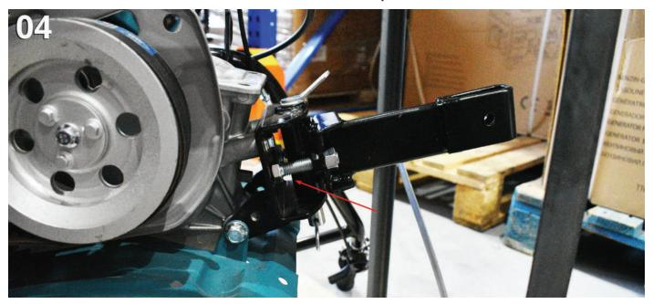
Fig. 5. Mount the transport wheel on the cultivator frame. Secure the wheel with a locking pin and cotter pin.
