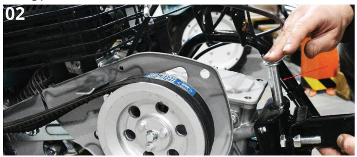
Fig. 3. Secure the locking pin with a cotter pin.
