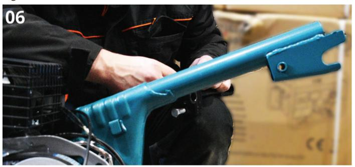
Fig. 7. Lock the position of the control handle with the clamp fixture.
