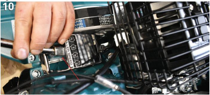
Fig. 11. Secure the shift lever extension with a locking pin, and then secure the locking pin with a cotter pin.
