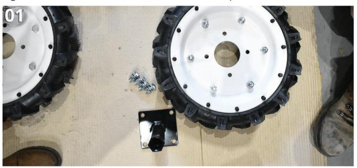
Fig. 2. Secure the transport wheel to the axle using bolts, nuts and washers.
