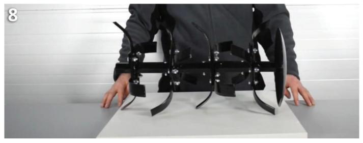
Fig. 9. The right cultivator cutters are mounted inversely. The cutting edge of the knives should be at the front in the direction of travel of the cultivator.
