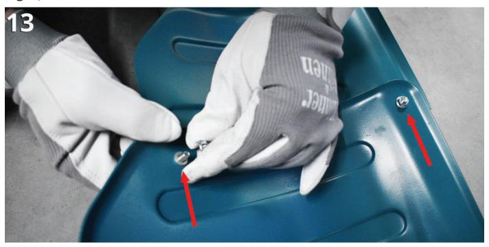
Fig. 14. Fasten the fenders to the cultivator body with screws.
