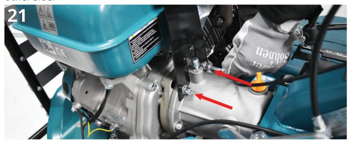
Fig. 22. Attach the guard top to the support foot using a bolt and nut.
