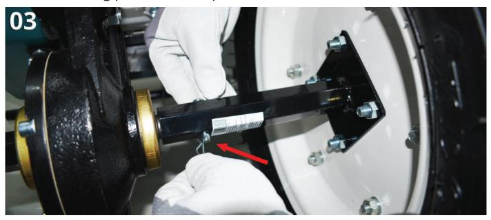
Fig. 4. Install the plow holder mount on the cultivator frame with the locking pin.
