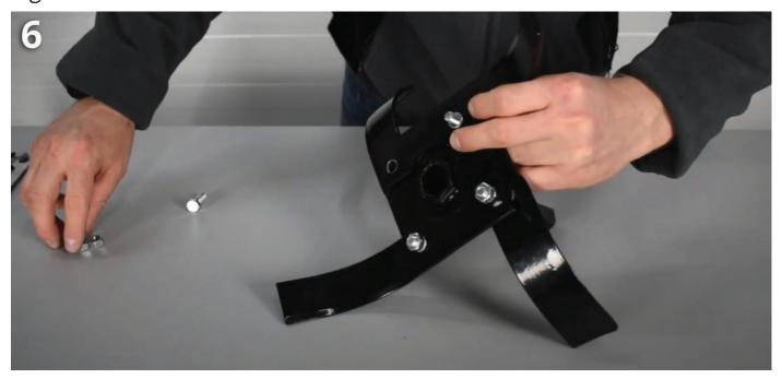
Fig. 7. Connect the sections together using locking pins, and then secure the locking pins with cotter pins.
