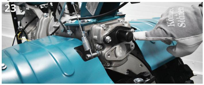
Fig. 24. Slide the semiaxle with cutters\* onto the gearbox shaft and secure with the locking pin.
