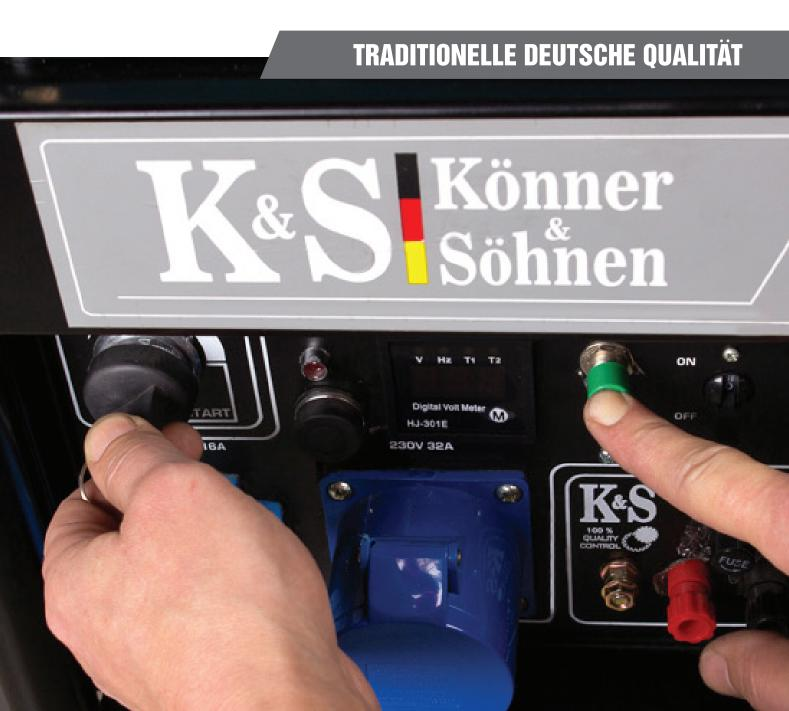
To start the generator in winter, turn the start key to the "START" position by holding the "HEAT" heating button on the generator panel.
