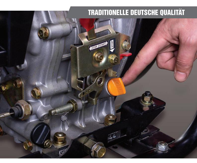
Before the first start, fill the crankcase with engine oil.
