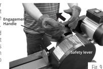
**If the Ram stops** before the end of the stroke while splitting a tough Log, quickly actuate the Engagement Handle back to the Auto-Retract position. Let the Ram return and allow the Flywheels to gain momentum for another full power split.
