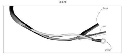
Each cable of the KS PU1 generator parallel connection box has three wires: red, black and yellow: The red wire is connected to the red connector on the generator control panel ("+" to "+"); the black wire is connected to the black connector on the generator control panel ("-" to "-"); and the yellow wire is connected to the ground terminal.
