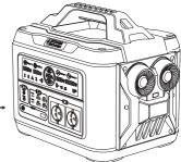
**Charging by DC input or Anderson 1 (18V~30V, 8A max/200W):** The icon  $\stackrel{\frown}{=}$  will lights up, show the current input power in watts input, and the percentage of the battery.
