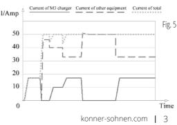
for the current drop of other equipment, Smart load controller KS SLC will control the KS X-Series (KS X32/1, KS X16/3, KS X32/3) current to rise slowly.
