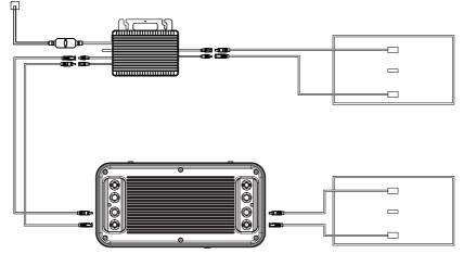
\*This issue arises from the fact that some of the microinverters available on the market have a common internal reference point. When both microinverter inputs are connected to a battery simultaneously, the microinverter will function abnormally.
