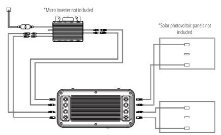
If you find that the microinverter is not functioning properly after the connection described above, please connect as follows: Connect one of the microinverter inputs to the DC MC4 Output of the battery, and the other microinverter input should either be disconnected or connected to the solar panel.
