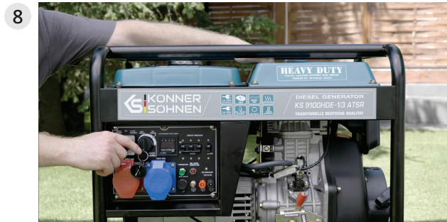
Turn the start key to "START" and hold it in this position for a few seconds. After 2-3 seconds, release the compression release lever without releasing the start key. After the engine starts, release the start key for it to return to "ON".
