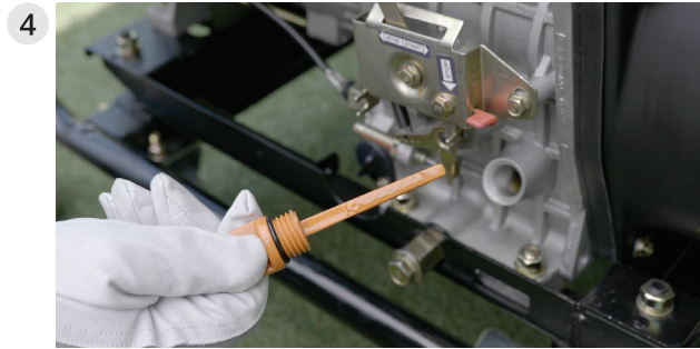
Information about the recommended amount of oil can be found in the manual. The oil level should be equal to the level in the filler neck. Make sure the oil level is between the MIN and MAX marks on the oil dipstick.
