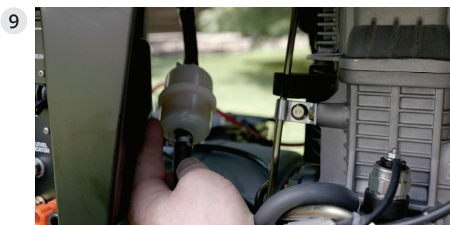
Air can get into the fuel system of the diesel generator, which can cause start-up complications. Therefore, if the generator does not start, you must perform the following steps: Look at the fuel filter, it may not be completely filled with fuel. Take the filter in your hand and try to remove air from it by changing its position (horizontally / vertically). Then try starting the generator again.
