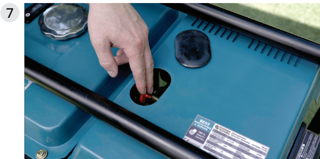
Remove the protective rubber plug on the top of the generator. Hold down the compression release lever.
