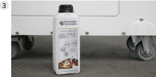
Fill the engine with motor oil for four-stroke diesel engines SAE 10W-30 or SAE 10W-40.
