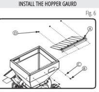
1. Hold the hopper guard assembly (A) so that the rubber guard is directed down towards the bottom of the hopper. Align the assembly holes with the holes in the hopper.
