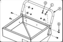
Hold the hopper handle (A) up so that the outer holes in the handle align with the holes in the hopper and secure with four M6 x 30, M6 washers (C) and M6 nuts (D). Insert the screws from the outside of the hopper.
